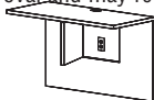
(1) 18"W x 15"H Door for Bridges, Returns, Single Pedestal Credenzas, and Kneespace Credenzas
